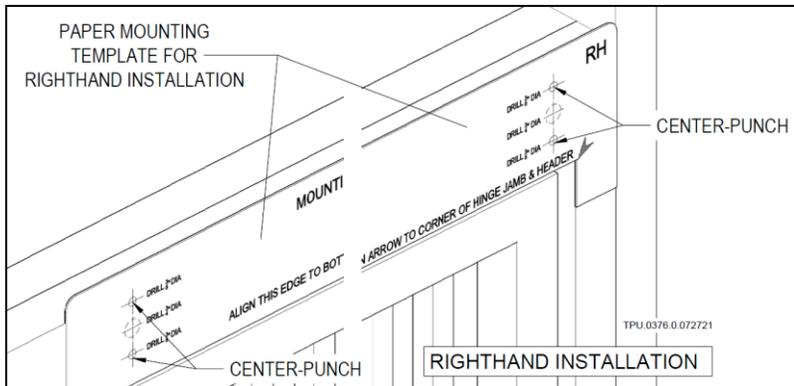
**STEP 4** Drill 1/16" pilot holes on header through Template
