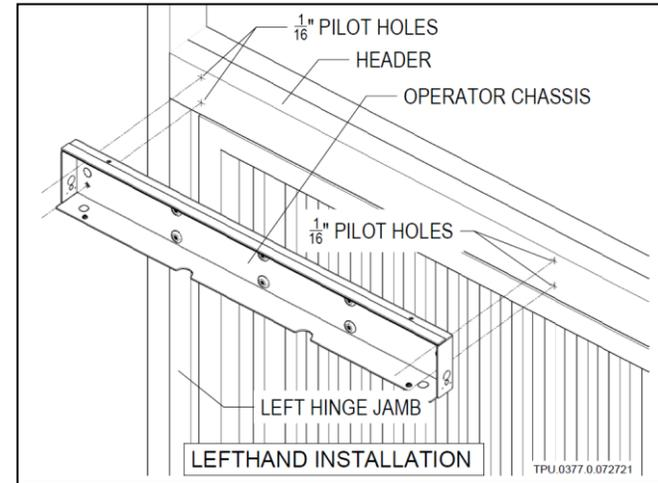
**STEP 6** Mount<sup>2</sup> Motor-Drive assembly to operator Chassis
