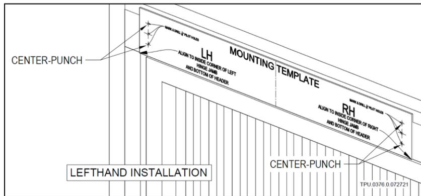
**STEP 4** Drill 1/16" pilot holes on header through Template
