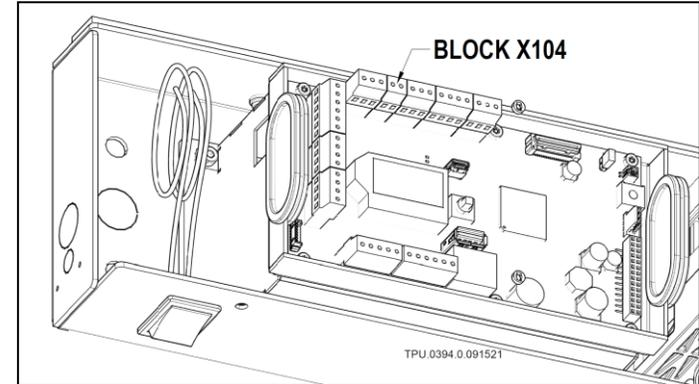
**STEP 4** Feed the switch wires through the rubber grommet on the control unit and connect to Block X104
