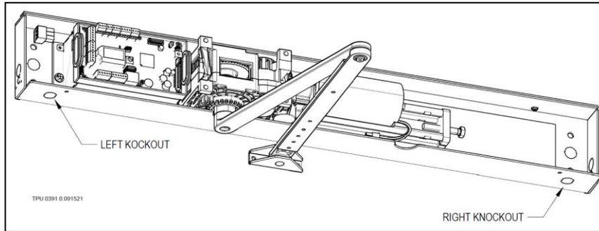
**STEP 1** Choose and punch out one knockout at the bottom of the AUTOPED chassis (Note: The following illustrations show the use of the left knockout)
