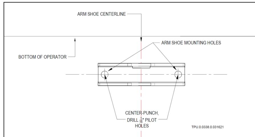
**STEP 6** Drill 1/16" pilot holes on the center marks
