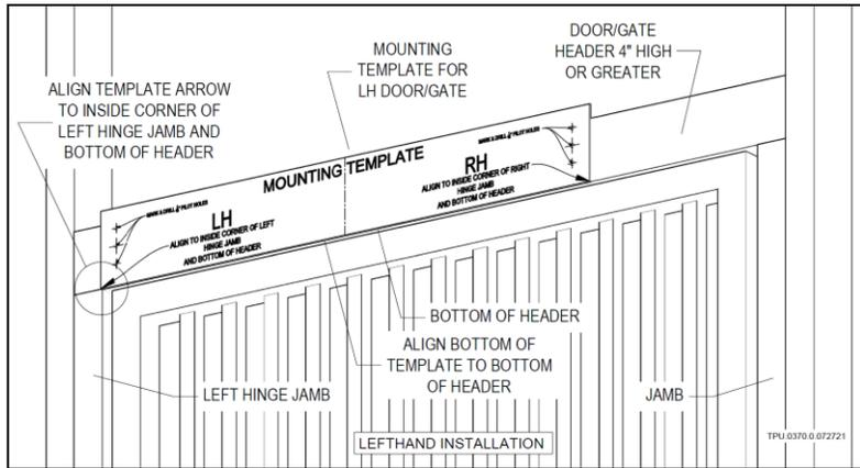
**STEP 3** Center-punch mounting holes through Template
