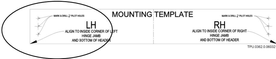
**STEP 2** Align arrow to inside corner of left hinge jamb and bottom of header
