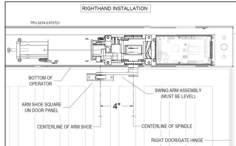
**Note:** Make sure the Swing Arm is inserted to the Gear Box snugly and installed level
