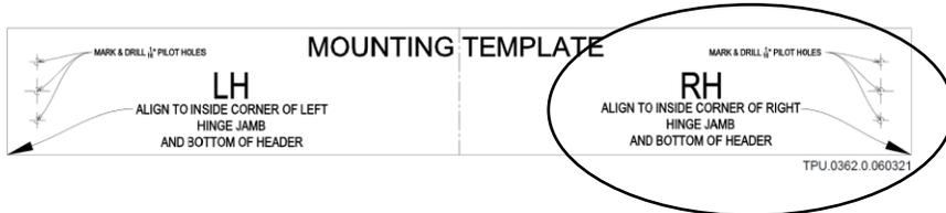
**STEP 2** Align arrow to inside corner of right hinge jamb and bottom of header
