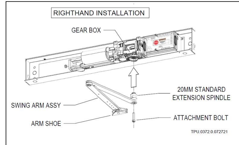
**Note:** A 30mm Spindle Extension is included in an optional kit (P/N M10S-0018), if needed, it may be used instead of the 20mm to lower further the Swing Arm assembly to have a wider clearance between bottom of AUTOPED operator and top of Arm Shoe
