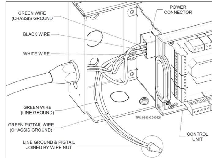
**STEP 6** Plug Power Connector back to Control Unit; turn AC power back on
