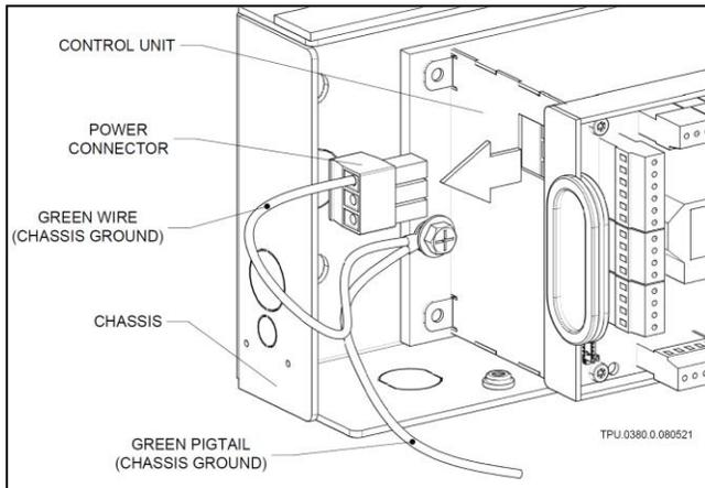
**STEP 3** Feed the 115 VAC line through a Wire Access Hole
