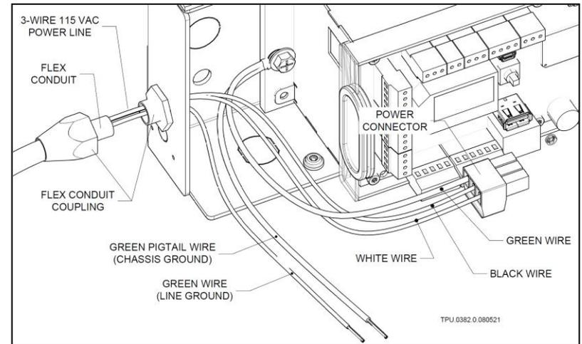
**STEP 5** Use wire nut to connect Line Ground and Green Pigtail wires together
