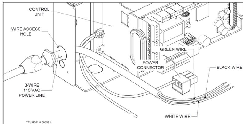
**STEP 4** Connect the 115 VAC wires to the Power Connector
