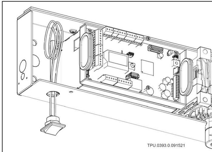
**STEP 3** Locate terminal Block X104 as shown in the figure below, and remove jumper across
