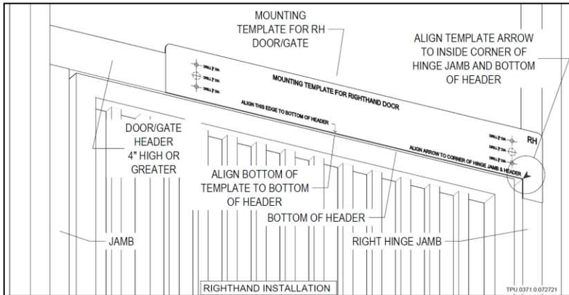
**STEP 3** Center-punch mounting holes through Template
